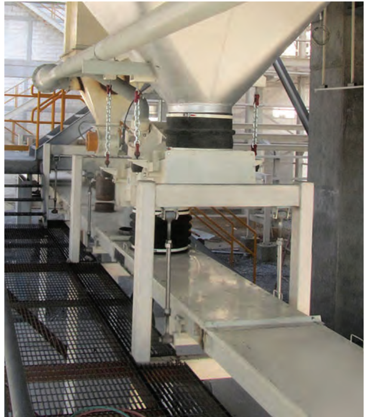
Horizontal motion conveyors replaced belt conveyors for a more dust free environment.
