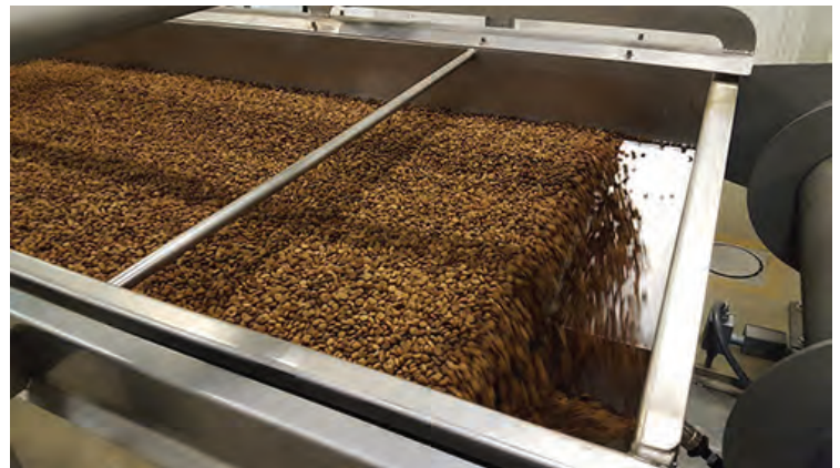
Horizontal motion conveyors replaced belt conveyors to provide a cleaner and safer solution for this pet food maker.
