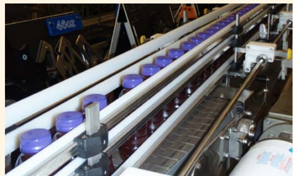
▶ Campbell Soup V-8® V-Fusion beverages in 12-ounce PET bottles move down the line on a new conveyor with adjustable rails. Source: Campbell Soup.
